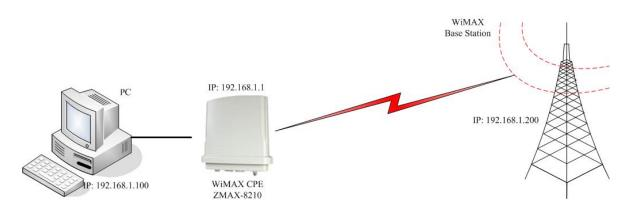
Figure 11 Build the Infrastructure with WiMAX Base Station
